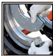
Inserts Ø 90 ÷ 280mm master Ø 250 mm
